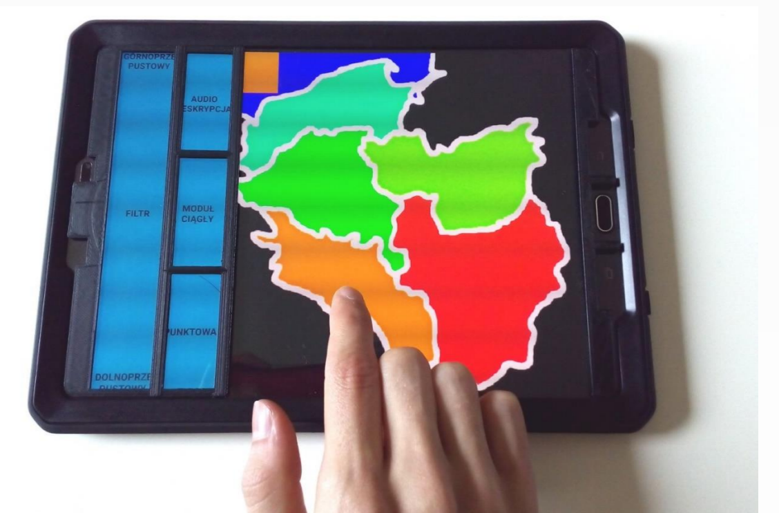
Custom 3D printed frames allow easier access to menu controls for blind users
